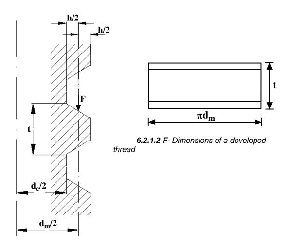
6.2.1.1 F- Loading and bending stresses in screw threads
